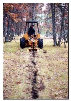
Vibratory Plowing (Figure 19): Manv miles of oak wilt areas in Michigan have been treated with a vibratory plow pulled behind a large tractor, following the perimeter line delineated around the epicenter. The plow has a blade that slices into the ground, at least five feet deep. facilitated by a powerful vibration action. Plowing must be at least five feet deep to ensure the oak roots are severed. Vibratory plowing should be done during the dormant season.
